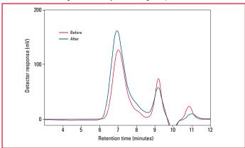
Figure 2. GPC elution profile for a polymer before and after temperature cycling obtained using a TSKgel GMH<sub>HR</sub>-H(S) HT column
