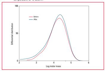
Figure 4. Overlay of the differential molar mass distribution of a polymer before and after temperature cycling obtained using a TSKgel GMH<sub>HR</sub>-H(S) HT column
